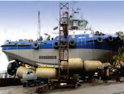
Draft reduction for newly constructed tugboat launching using Salvage Pontoons 40,000 lbs. and Salvage Pontoons 70,000 lbs.
