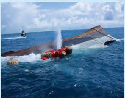
Raising the Spiegel Grove, a 510 ft U.S. Navy troop transport ship.
