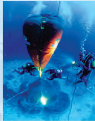
Professional 4,000 lbs. Lift Bags raising 5 ton marble column sections from a 200 BC Roman shipwreck off of Turkey
